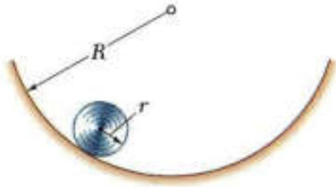
Determine the period of small oscillations of a cylinder which rolls without slipping inside a curved surface.
