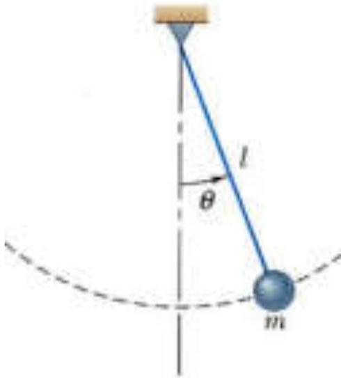
Results obtained for the spring-mass system can be applied whenever the resultant force on a particle is proportional to the displacement and directed towards the equilibrium position.
