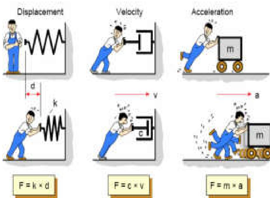
All mechanical systems can be modeled by containing three basic components:
