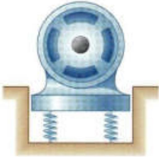
A motor weighing 350 lb is supported by four springs, each having a constant 750 lb/in. The unbalance of the motor is equivalent to a weight of 1 oz located 6 in. from the axis of rotation.
