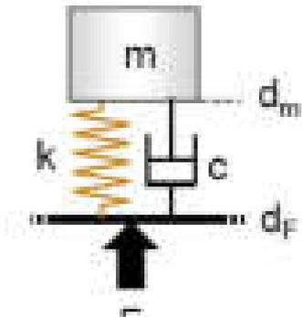
If an external force applied to a system, the system will follow the force with the same frequency.
