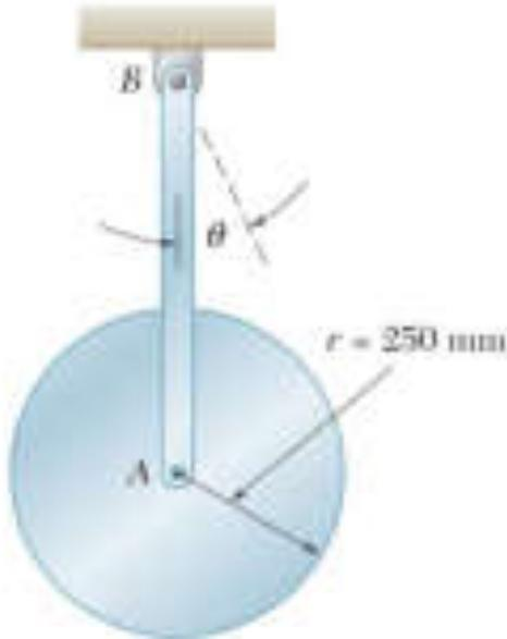
A uniform disk of radius 250 mm is attached at  $A$  to a 650-mm rod  $AB$  of negligible mass which can rotate freely in a vertical plane about  $B$ . If the rod is displaced  $2^\circ$  from the position shown and released, determine the period of the resulting oscillation.
