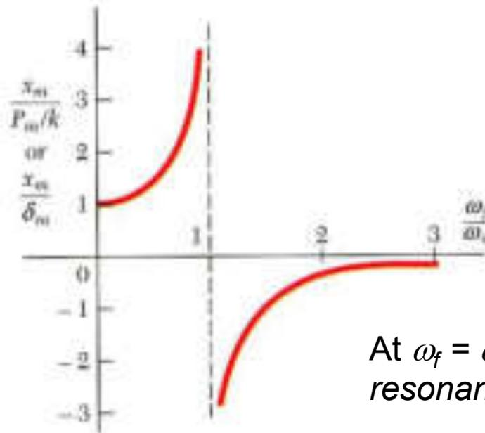
At  $\omega_f = \omega_n$ , forcing input is in *resonance* with the system.
