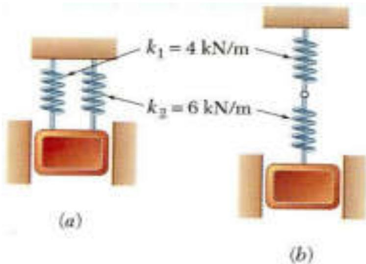
A 50-kg block moves between vertical guides as shown. The block is pulled 40mm down from its equilibrium position and released.
