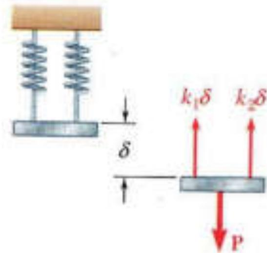
$$\omega_n = \sqrt{\frac{k}{m}} = \sqrt{\frac{10^4 \text{ N/m}}{20 \text{ kg}}} = 14.14 \text{ rad/s}$$
