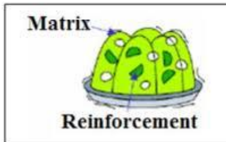
Fig 1 Matrix and Reinforcement in a Composite Material
